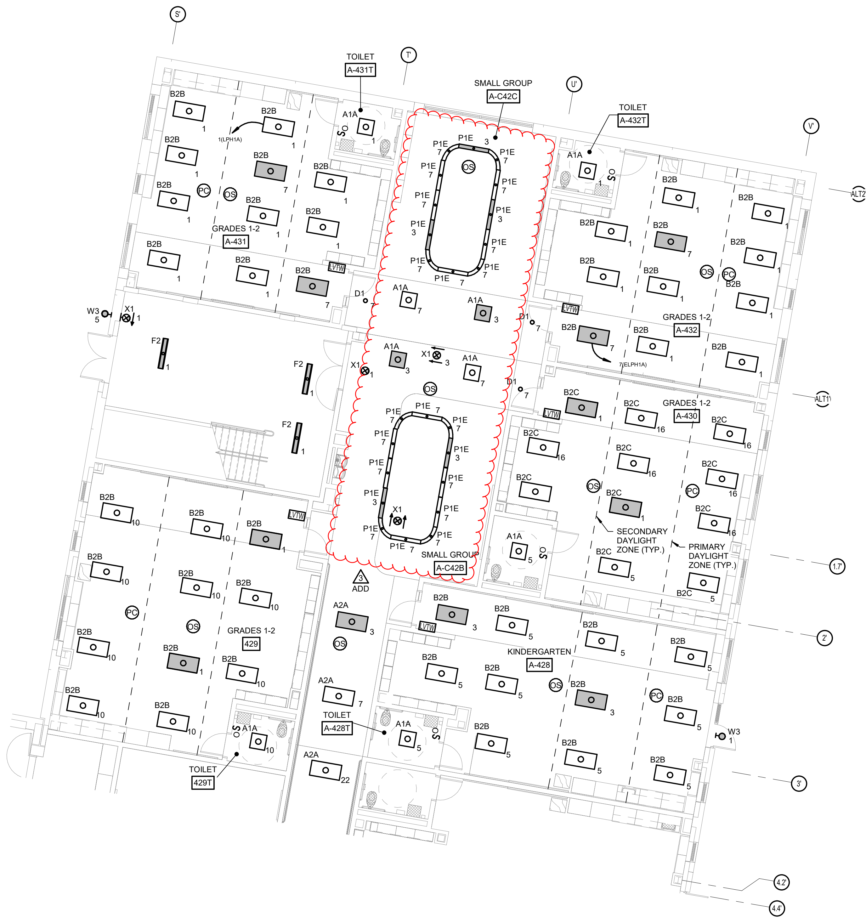
1 PART FIRST FLOOR PLAN - LIGHTING - ALTERNATE SCALE: 1/8" = 1'-0"
